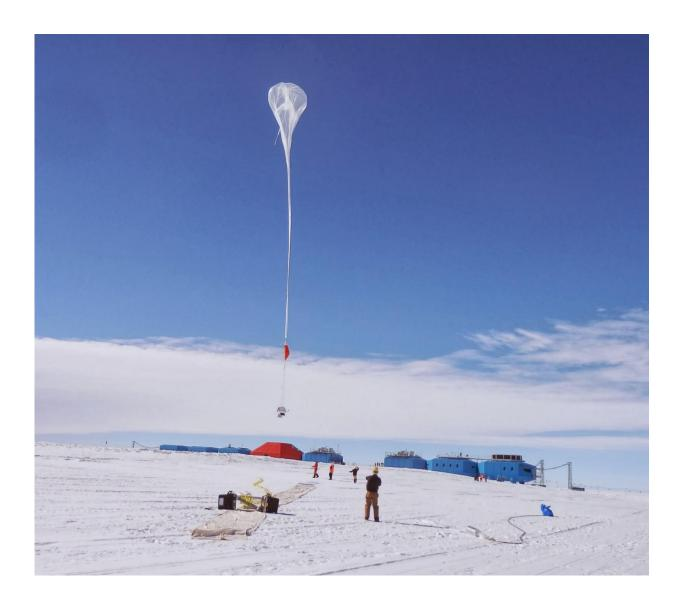
A BARREL balloon launches over Halley Research Station during the Antarctic summer of 2013-2014. The BARREL mission was created to observe precipitating electrons from Earth's radiation belts, supplementing observations
