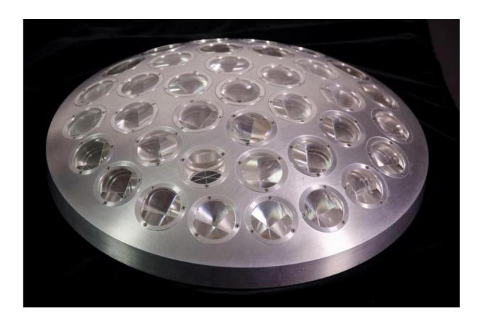
The surface of LAGEOS is dotted with 426 cube-corner prisms to reflect laser pulses transmitted from ground stations on Earth. One sector of a model is shown here. With LAGEOS, the accuracy of laser ranging measurements improved from about 3 feet (1 meter) to less than half an inch (1 centimeter). Credit: NASA's Goddard Space Flight Center
