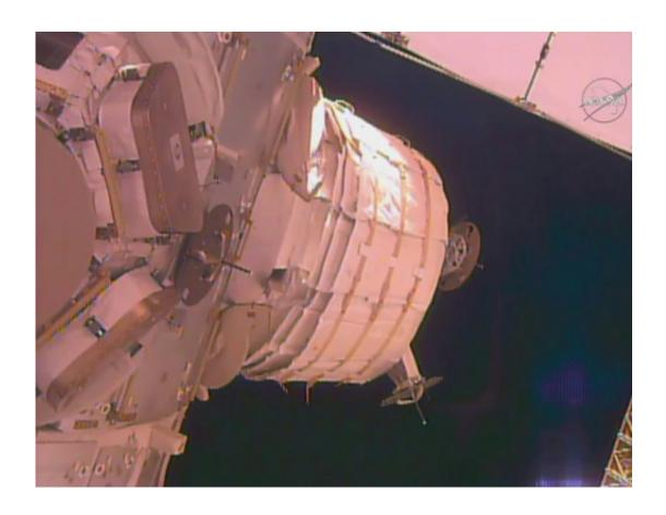
The unexpanded Bigelow Expandable Activity Module seen attached to the Tranquility module of the International Space Station on May 26, 2016
