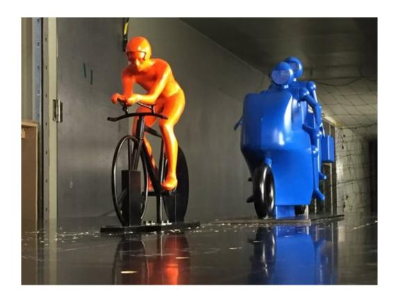
Scale models used for the wind tunnel measurements. Credit: Eindhoven University of Technology
