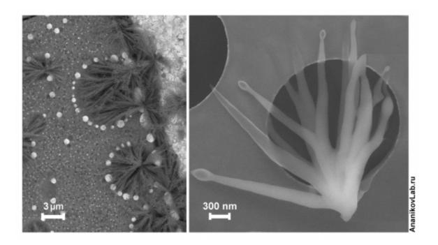
Cryogenic scanning electron microscopy study of solution phase of catalytic cross-coupling reaction. Credit: AnanikovLab.ru
