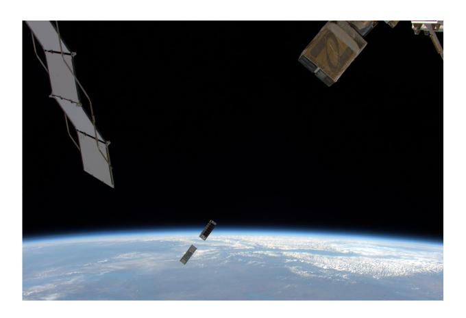
On May 16, 2016, the NASA-funded MinXSS CubeSat deployed from an airlock of the International Space Station to enter an orbit around Earth. MinXSS observes soft X-rays from the sun -- such X-rays can disturb the ionosphere and thereby hamper radio and GPS signals. Credit: ESA/NASA
