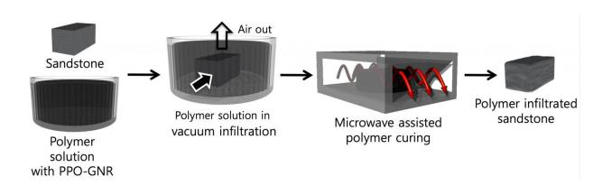
Rice University researchers have developed a method to treat composite materials of graphene nanoribbons and thermoset polymers with microwaves in a way that could dramatically reinforce wellbores for oil and gas production. Credit: Nam Dong Kim/Rice University
