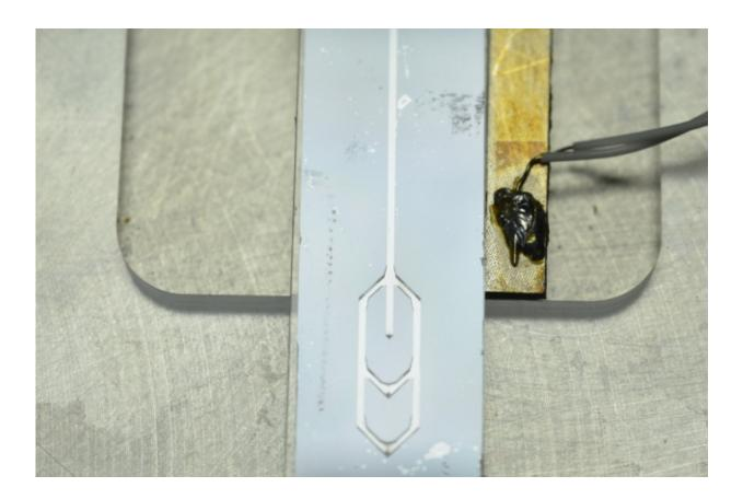
A new cell-sorting device consists of a microfluidic channel that vibrates at a very low frequency. As cells flow through the channel, they are pushed to a certain position depending on how they interact with the acoustic forces generated by the vibration. Pictured is an example of the device.
