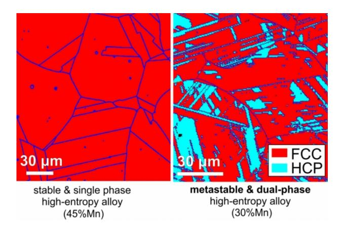
These images show the crystal configurations, or phases, within samples of metal alloys: a single-phase stable alloy (left) and a dual-phase alloy (right), which is metastable (has more than one stable configuration). The dual-phase material turns out to have better strength and ductility than the singe-phase material, the researchers found.
