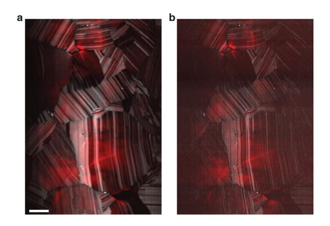
Photoluminescence (red) and second harmonic generation (grayscale) from pure cadmium-telluride solar cells, imaged simultaneously. Standard resolution is on the left, and enhanced resolution, on the right, was captured by a CSU custom-built microscope. Credit: Jeffrey Field/Colorado State University
