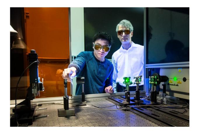
Adrian Sabau and Jian Chen work with a laser to prepare the surface of carbon fiber composites and aluminum to create superior bonds that can absorb 200 percent more energy than conventional bonds. Credit: ORNL
