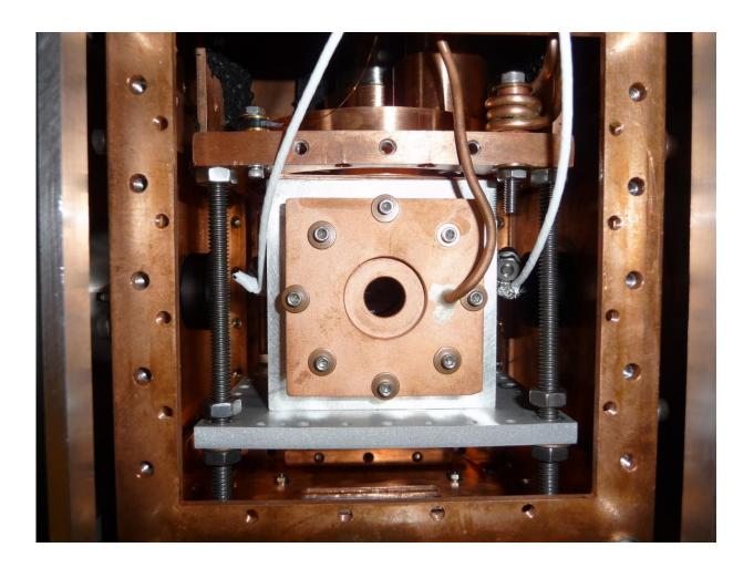
JILA instrument that uses a frequency comb to detect large, complex moleculesbased on the precise frequencies, or colors, of light they absorb. Themolecules are chilled and probed inside this chamber at temperatures nearabsolute zero. Credit: Spaun/JILA
