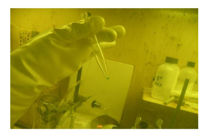
The green dot at the bottom of the glass vial is a solution containing 22 milligrams of ultra-pure <sup>249</sup>Bk produced at ORNL's High Flux Isotope Reactor and Radiochemical Engineering Development Center at ORNL.
