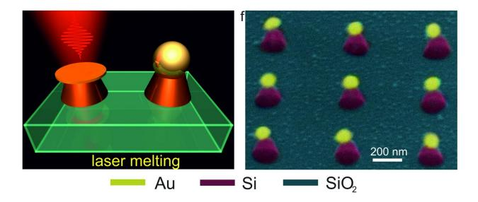
SEM image of fabricated nanoantennas. Credit: ITMO University
