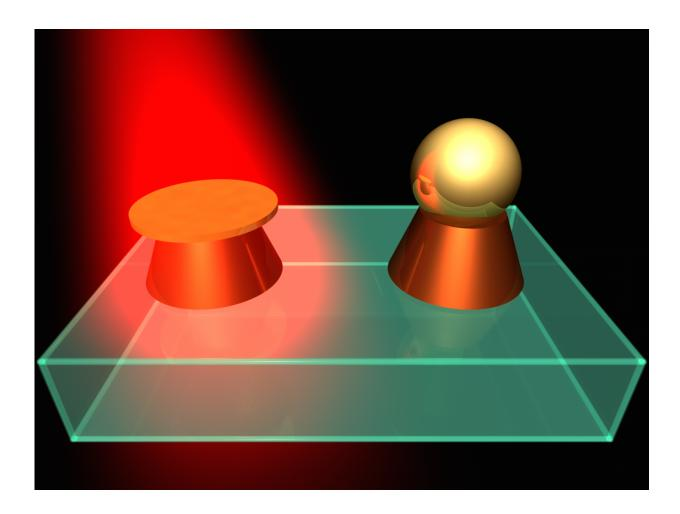
Selective laser exposure to create hybrid nanostructures. Credit: ITMO University
