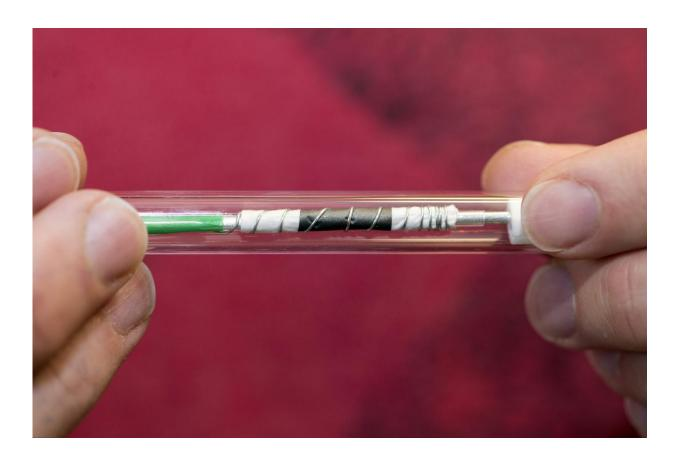
Corresponding author Johannes Wandt with one of the electron paramagnetic resonance probes he developed for the detection of singlet-oxygen which is produced during the charging process. Credit: Andreas Battenberg / TUM
