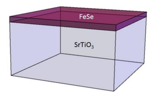
A schematic drawing of an atomically thin FeSe film grown on SrTiO3 substrate. Credit: ©Science China Press
