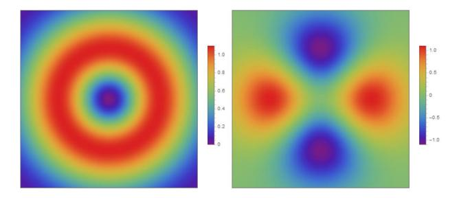
Cooper pair wavefunctions with different symmetry. On the left the sign of the wavefunction remains the same under 90o rotation while the sign reverses for the wavefunction on the right. Credit: ©Science China Press
