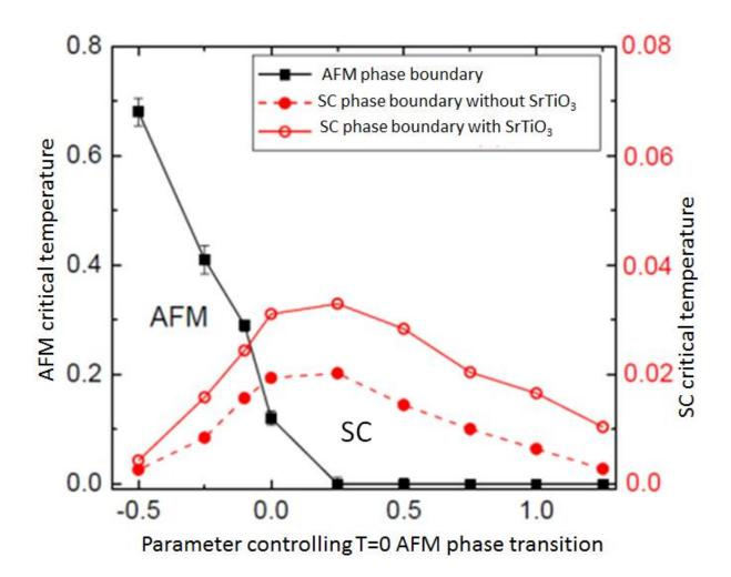
The phase diagram deduced in Ref.[1]. The black symbols mark the phase boundary of the 'antiferromagnetic' order and the red ones mark the superconducting transition. The open and solid red circles refer to the presence and absence of electron-phonon interaction. In the absence of SrTiO3 it is a magnetic interaction that causes the formation of Cooper pairs. Credit: ©Science China Press
