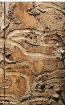
Solid wood packaging materials, such as pallets and crates, are the fastest-growing source of highly damaging pests. An inspector examines solid wood packaging (left). The Emerald ash borer larva creates a "carving gallery" in the wood (right). Credit: (left) USDA; (right) John Hritz
