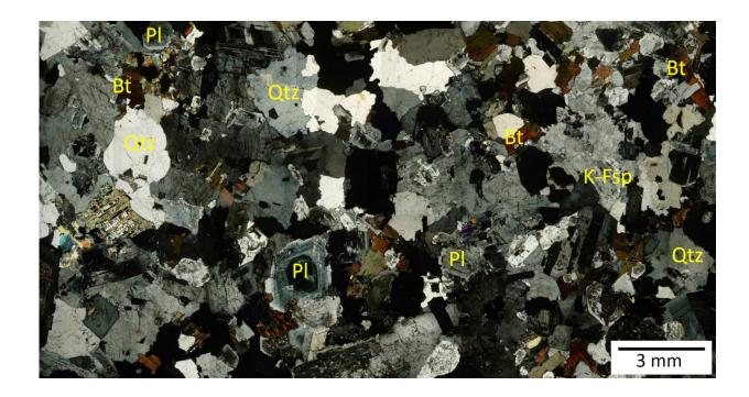
Alpedrete granite seen under a petrographic microscope. The main minerals are indicated: quartz (Qz), potassium feldspar (K-Fsp), plagioclase (Pl) and biotite (Bt). Credit: D. M. Freire-Lista/IGEO (CSIC-UCM)
