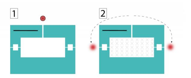
Three superconducting islands (teal) surround a rectangular hole. One island supports a thin semiconductor wire. As a magnetic field is turned up in the central region, a single magnetic vortex is coaxed into the empty area. The path that the vortex takes is indeterminate and leads to a quantum interaction between the vortex and a qubit stored by the wire.
