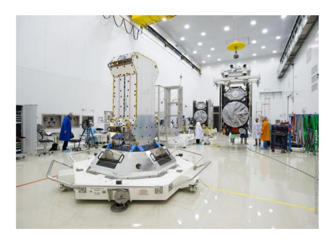
Europe's 13th and 14th Galileo satellites undergoing a fit check with their dispenser in the S1A cleanroom facility in mid-April 2016. The satellites were mechanically and electrically linked to the dispenser ahead of fuelling, after
