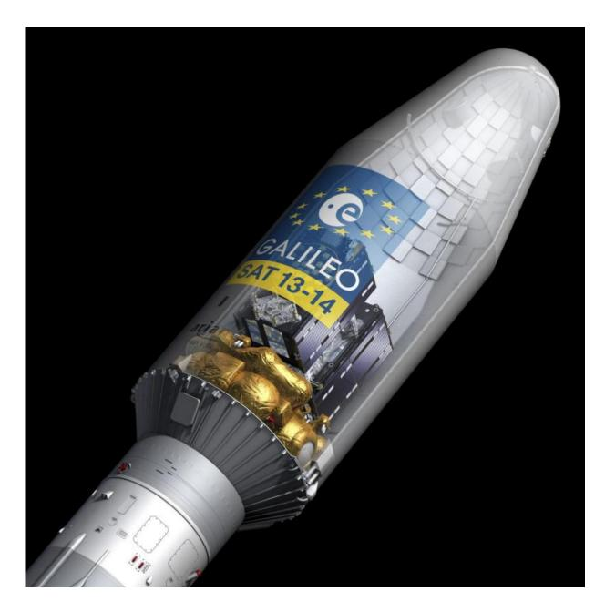
Cutaway view of the Soyuz rocket fairing carrying the Galileo-13 and -14 satellites, seen atop the Fregat upper stage that will fly them most of the way to their intended medium-altitude orbit. Credit: ESA–Pierre Carril, 2016
