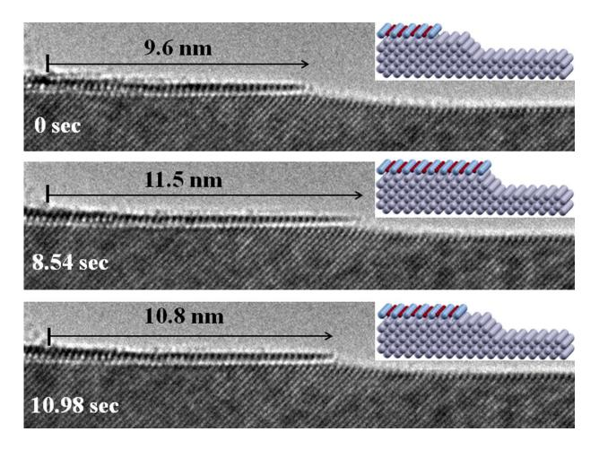
An in-situ atomic-scale observation of the oxidation process of a copper surface by transmission electron microscopy. Credit: Guangwen Zhou
