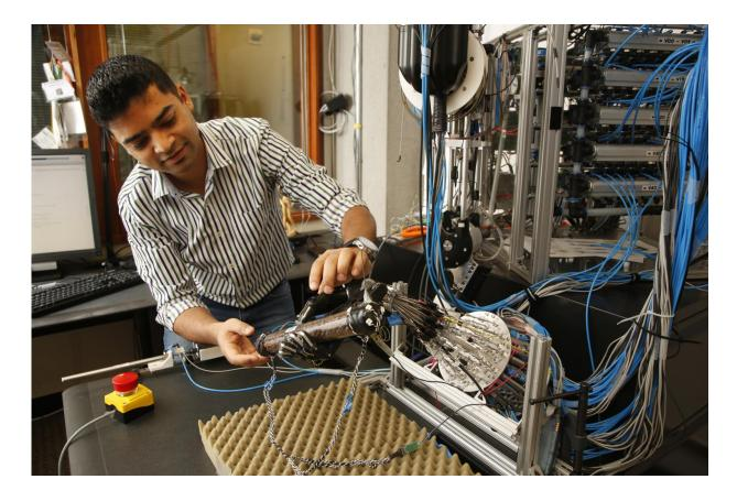
UW computer science and engineering doctoral student Vikash Kumar developed this robot hand actuated with a custom pneumatic system. It has 40 tendons, 24 joints, more than 130 sensors and can move faster than a human hand. Credit: University of Washington
