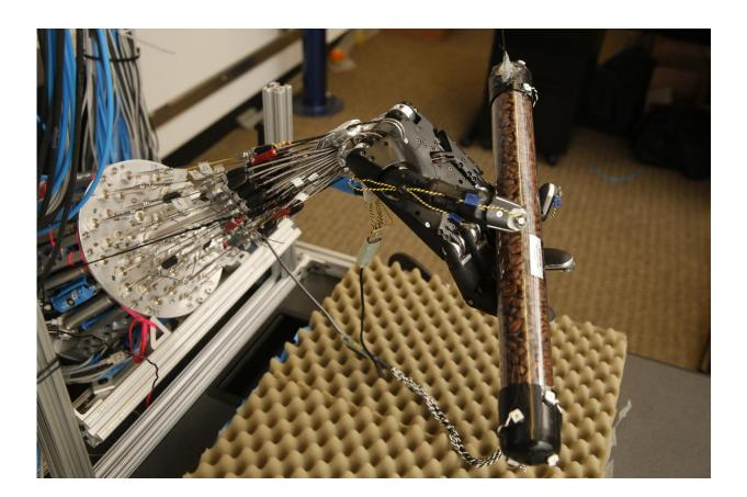
This five-fingered robot hand developed by University of Washington computer science and engineering researchers can learn how to perform dexterous manipulation -- like spinning a tube full of coffee beans -- on its own, rather than having humans program its actions. Credit: University of Washington
