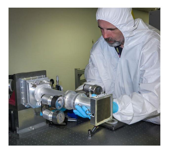
Target Diagnostics Facility technician Glen Grant mounts a large-aperture proton radiography imaging diagnostic on the snout of a diagnostic instrument manipulator for a collisionless shock experiment.
