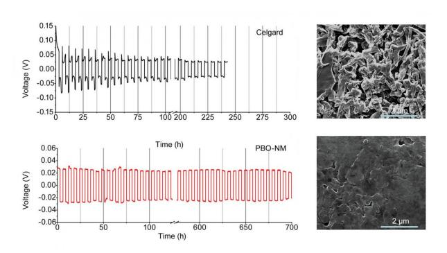
(Top) The voltage of a battery with the Celgard 2400 membrane separator decreases over time. Dendritic lithium is visible on the electrode surface after 230 hours of cycling. (Bottom) The voltage of a battery with the new Zylon membrane separator exhibits long-term stability. After 700 hours of cycling, the lithium surface remains smooth and dendrite-free. Credit: Hao et al. ©2016 American Chemical Society
