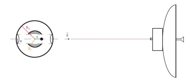
In the proposed experimental setup, a host spacecraft (right) shines a femtosecond laser pulse onto a retroreflector moving in the tunnel of a sphere (left). The period of the retroreflector's harmonic motion provides information on the value of G. Credit: Feldman et al. ©2016 IOP Publishing
