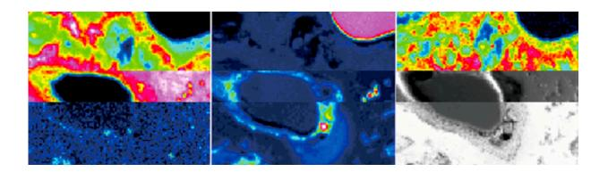
Compilation of control rod cross-sectional images, showing results of high-temperature steam oxidation.
