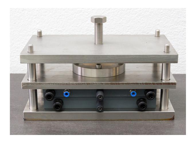
In this electrolytic cell Fraunhofer researchers produce hydrogen peroxide with electricity for local use – just from air and water. Credit: Fraunhofer
