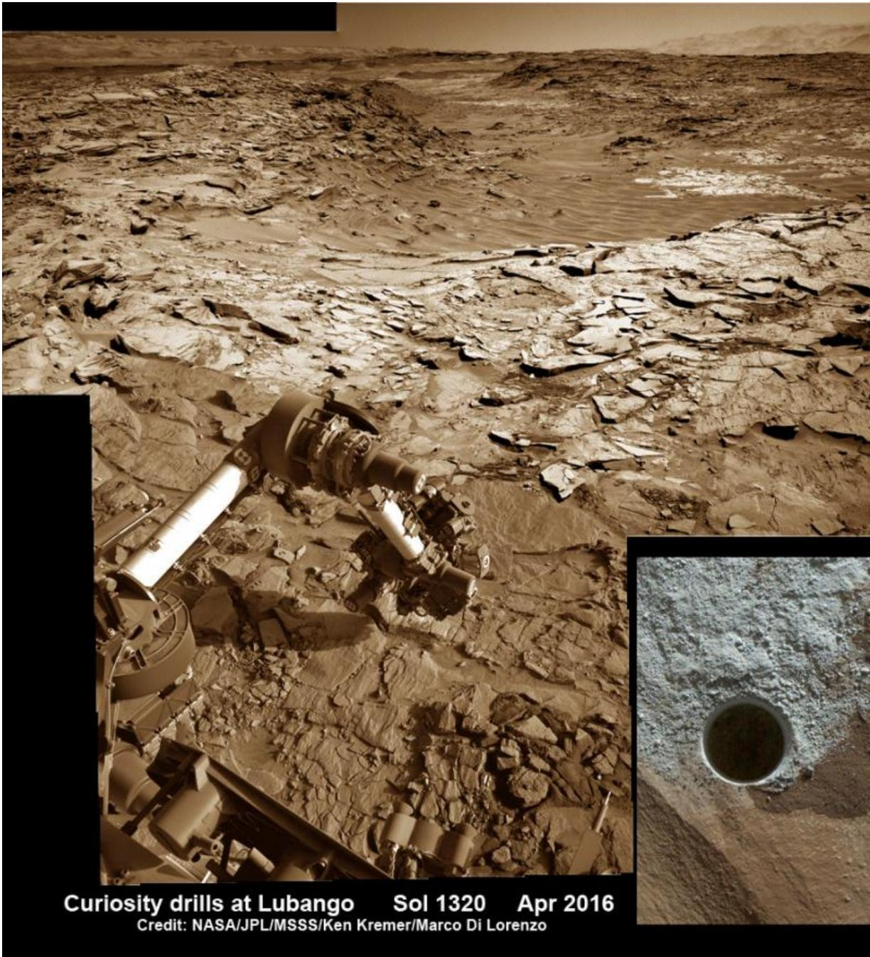
Curiosity rover reached out with robotic arm and drilled into ‘Lubango’ outcrop target on Sol 1320, Apr. 23, 2016, in this photo mosaic stitched from navcam camera raw images and colorized. Lubango is located in the Stimson unit on the lower slopes of Mount Sharp inside Gale Crater. MAHLI camera inset image shows drill hole up close on Sol 1321. Credit: NASA/JPL/MSSS/Ken Kremer/[kenkremer.com](http://kenkremer.com)/Marco Di Lorenzo
