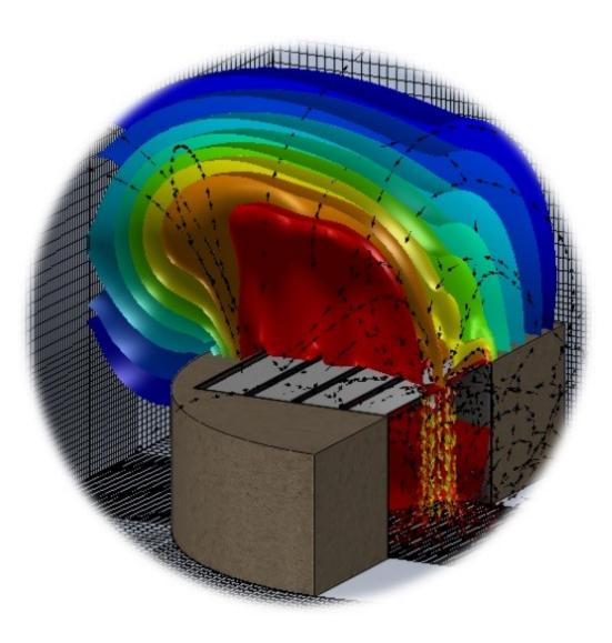
Storage pits commonly contain hydrogen sulfide, carbon dioxide, methane and ammonia. The online design tool, which pit designers and field engineers can use to predict and understand airflow in confined spaces -- depicted in this graphic -- is the culmination of a decade of research by a team of scientists in Penn State's
