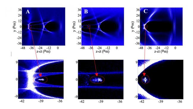
Researchers propose a new method to improve plasma wakefield accelerators by compressing the electron beam. Simulations show two-dimensional electron density distribution for the injector stage (A), compressor stage (B) and accelerator stage (C), where the target e-beam is circled by a dashed circle (in red). Credit: Jiansheng Liu/Chinese Academy of Sciences
