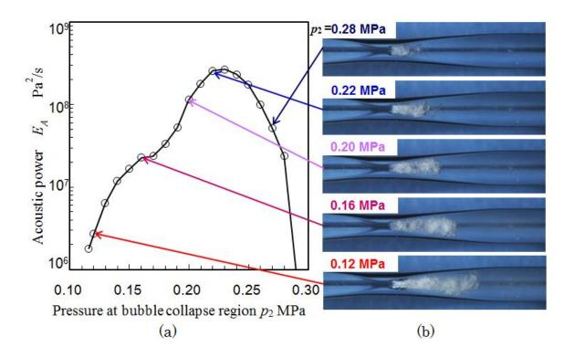
Although the developing region of hydrodynamic cavitation is decreased with an increase of pressure at bubble collapse region p2, the acoustic power is increased with the pressure and it has a peak at certain pressure. Credit: Hitoshi Soyama
