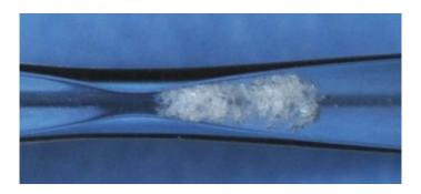
This image shows hydrodynamic cavitation through a venturi tube. Credit: Hitoshi Soyama
