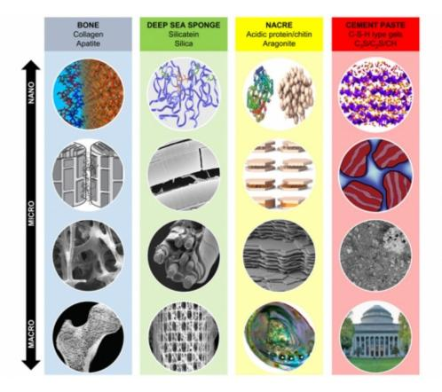
A comparison of natural materials and cement paste demonstrates the steps by which smaller pieces assemble to form larger structures.
