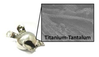
An innovative titanium-tantalum alloy can be printed into 3D shapes by selective laser melting for biomedical applications. Credit: A\*STAR Singapore Institute of Manufacturing Technology
