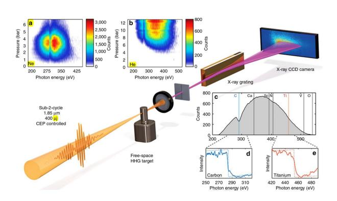
Experimental setup showing pressure dependence and spectral coverage. Credit: ICFO
