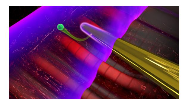
When laser light interacts with a nanoneedle (yellow), electromagnetic near fields are formed at its surface. A second laser pulse (purple) ejects an electron (green) from the needle, which can be used to characterize the near fields. Credit: Christian Hackenberger
