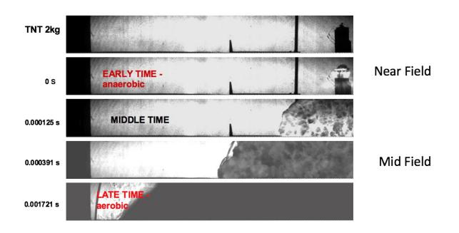
Horizontal view 2m across of a 2 kg TNT cylinder being top-detonated. The detonation products expand into air at a rate of several mm/usec, with a shock at the surface of the products (the explosive near-field). As air drag slows the detonation products, the shock detaches and travels through the ambient air - the explosive mid-field. Credit: McNesby/U.S. Army Research Laboratory
