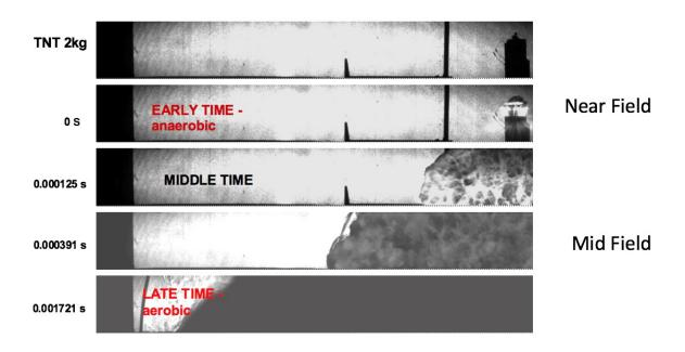
Horizontal view 2m across of a 2 kg TNT cylinder being top-detonated. The detonation products expand into air at a rate of several mm/usec, with a shock at the surface of the products (the explosive near-field). As air drag slows the detonation products, the shock detaches and travels through the ambient air - the explosive mid-field. Credit: McNesby/U.S. Army Research Laboratory
