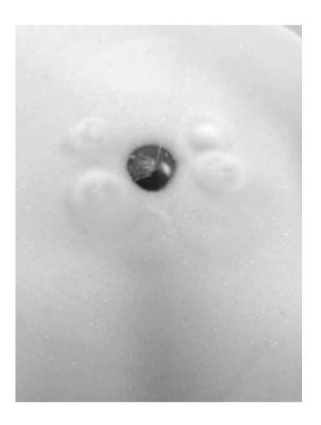
Sphere sinking in apparently fixed bed: Local bubbling around the spheres in density ratio ?1.3, whereas no bubble formations in density ratio >1.3. Credit: Okayama University, Osaka University, University of Melbourne and Swinburne
