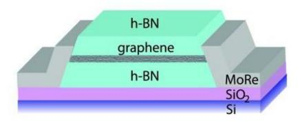
Illustration of the encapsulated graphene heterostructure with molybdenum rhenium contacts. Credit: (c) *Science* (2016). DOI: 10.1126/science.aad6203
