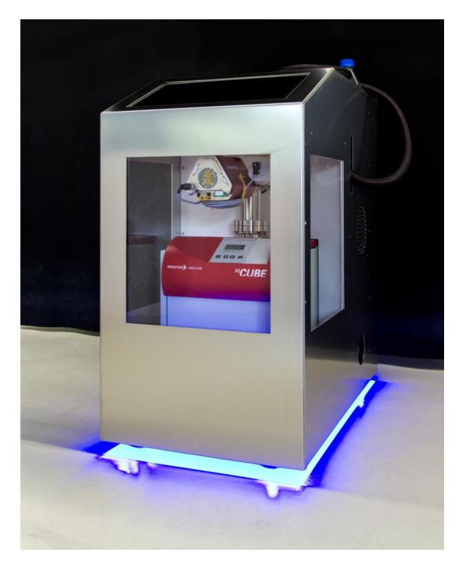
With this compact mass spectrometer up to 30 components can be analyzed simultaneously in the gas phase and a liquid.
