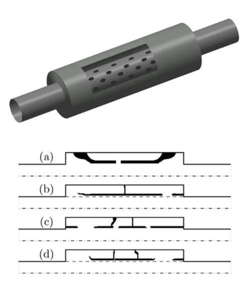
A cylindric muffler, about one meter long, at the start of the process. Below, the final muffler designs from topology optimization of a cylindrical symmetric reactive muffler for different target.
