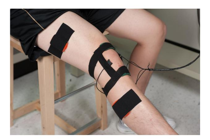
MEMS microphones and piezoelectric strips pick up sounds of a bending and extending knee. Professor Omer Inan is engineering a device to convert knee joint sounds into a signal he hopes medical researchers will be able to use. Credit: Fitrah Hamid / Georgia Tech
