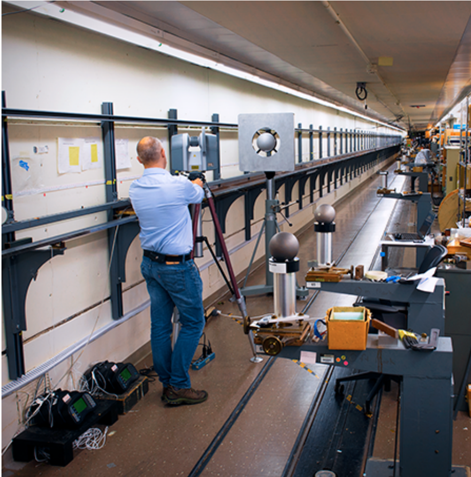
A participant performing relative range measurements in the long length tape tunnel facility at NIST. Credit: Sean Kelley/PML
