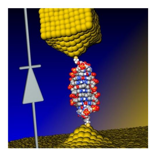
Illustration of the coralyne-intercalated DNA junction used to create a singlemolecule diode, which can be used as an active element in future nanoscale circuits. Credit: U. Georgia/Ben-Gurion U.
