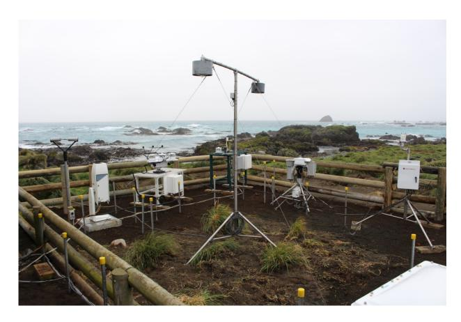
Instruments, installed in late March, will record just how cloudy it is in the Southern Ocean, how much sunlight reaches the surface, and how much water is in these clouds. Credit: Jeff Aquilina
