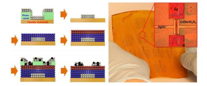
Because this entirely ink-based fabrication process works at lower temperatures than existing vacuum-based methods, the researchers were able to make several transistors on the same flexible plastic backing at the same time. Credit: University of Pennsylvania
