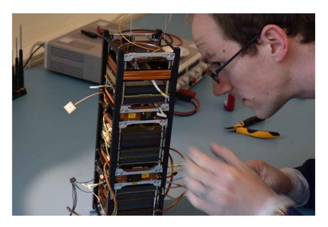
The technology-testing GomX-3 under construction. It was developed for ESA by GomSpace in Aalborg, Denmark, which is one of Europe's main CubeSat manufacturers. A 'three-unit' CubeSat, it measures 10x10x30 cm with an approximate mass of 3 kg, with payloads to detect signals from aircraft and telecom satellites. Credit: http://davidgerhardt.com
