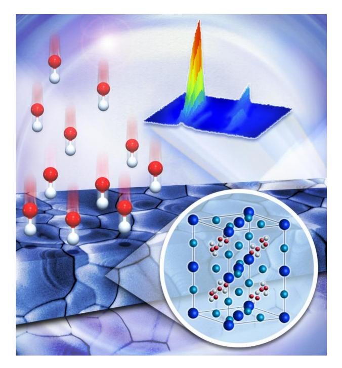
Oak Ridge National Laboratory scientists combined imaging techniques to measure crystallization kinetics of perovskite films following exposure to a mixed halide vapor. Over time, extra halide reactants settle in the film's grain boundaries, demonstrating atomic competition in crystal growth. Credit: Jill Hemman, Oak Ridge National Laboratory
