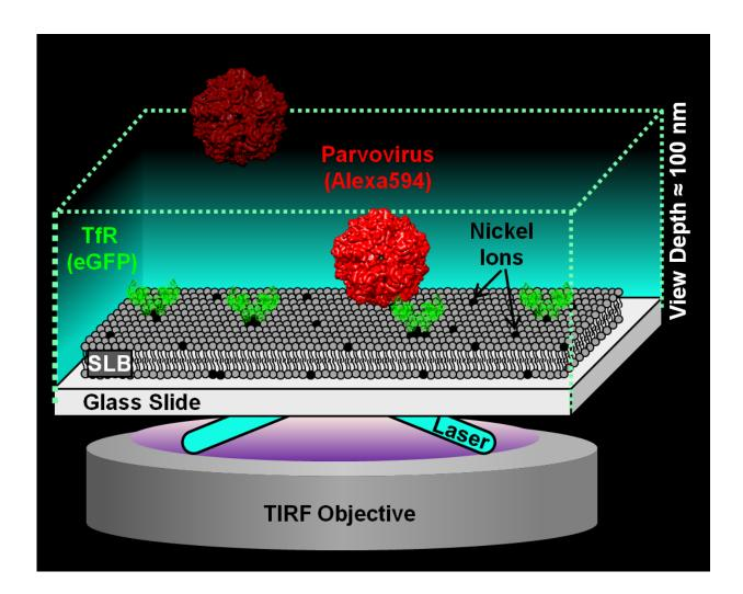
A schematic of the single-particle tracking binding as say used in the research in to parvovirus. Credit: Cornell University
