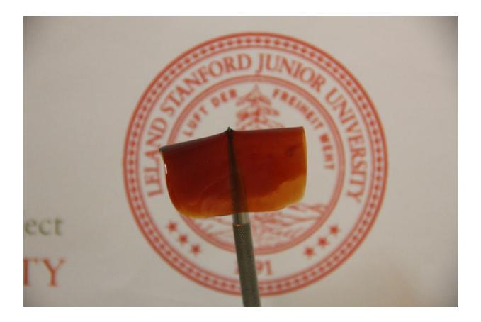
A new, extremely stretchable polymer film created by Stanford researchers can repair itself when punctured, a feature that is important in a material that has potential applications in artificial muscle. Credit: Bao Research Group
