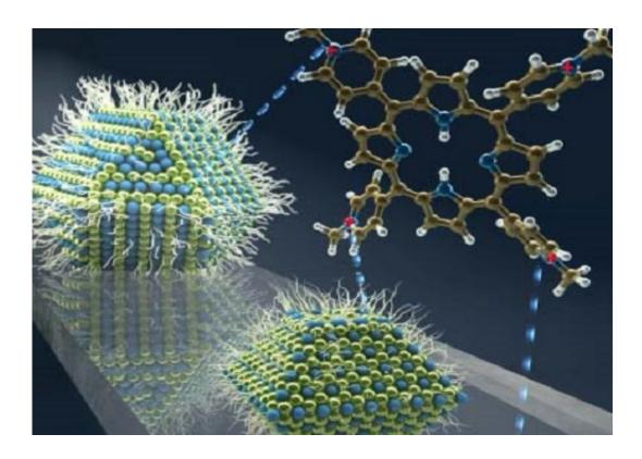
Organic molecules aid charge transfer from large lead sulfide quantum dots for improved solar cell performance. Credit: 2015 Wiley
